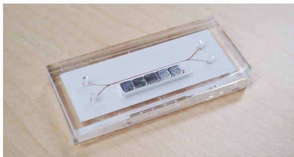
Figure A.6: Initial design with two inlets and outlets alongside a magnet array.
