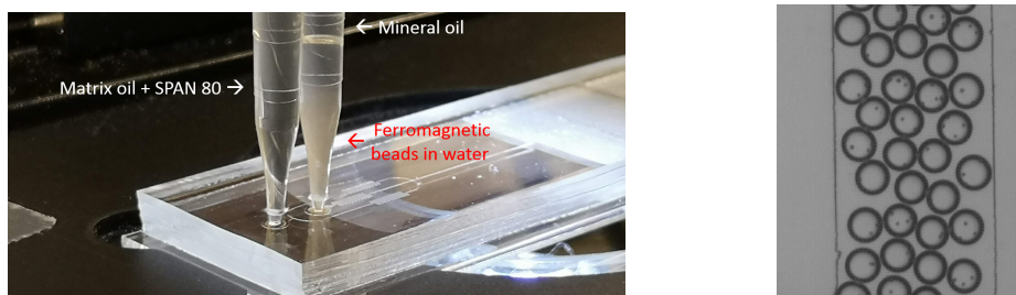
(a) Sedimentation of tip-loaded magnetic microparticles inside the right-hand pipette tip. Approx. 15 minutes into testing. (b) Droplets containing ferromagnetic microparticles.
