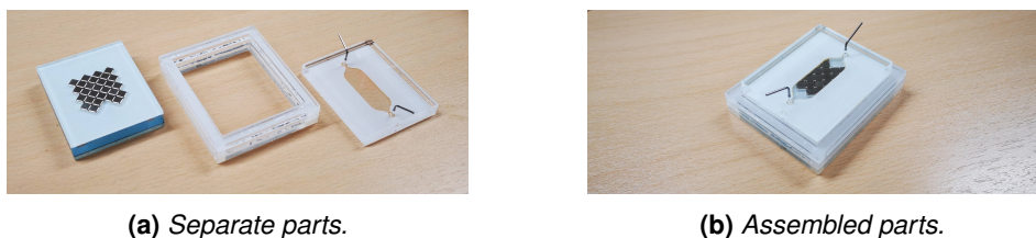
Figure 3.15: Magnetic platform, frame and the chip (including inlet and outlet needles)
