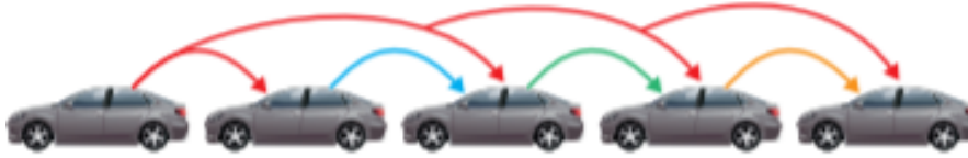
Figure 2.1: Vehicle-to-vehicle communication strategy to achieve collision-free driving and string stability [15]
