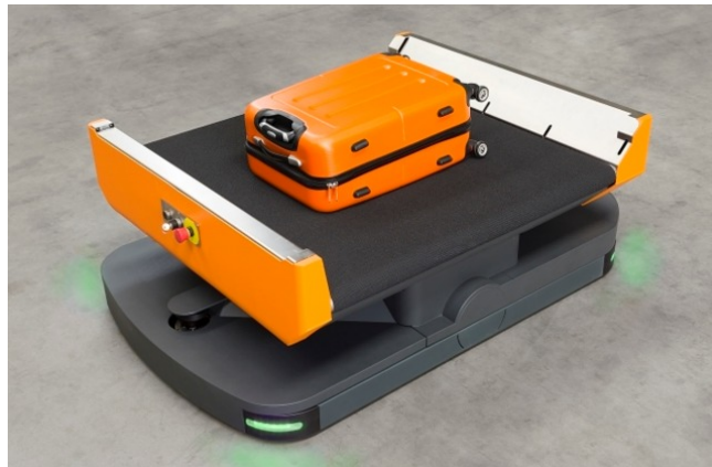
Figure 1.1: Example AGV used to transport baggage at airports. [4]
