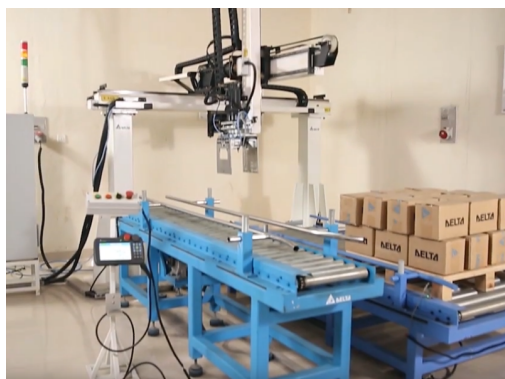
Figure 2.1: Example of a Cartesian (3PR) palletizing robot 1 .
