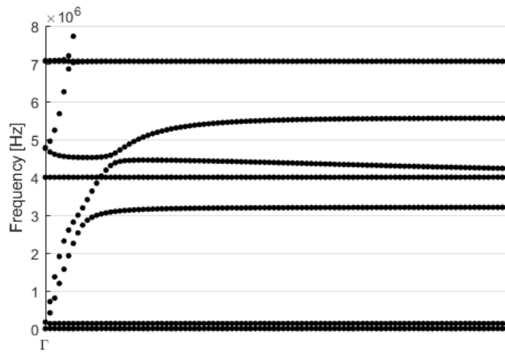
Figure C.2: Frequency band diagram of a double negative unit cell with a rotated incident wave of 20 degrees. The negative band has split.
