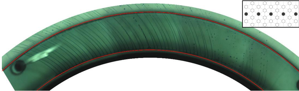
Figure 34. Example of an experiment with maldistribution of the fluid. It is clearly visible that the holes on right lack the water to produce similar jets as seen on the left.
