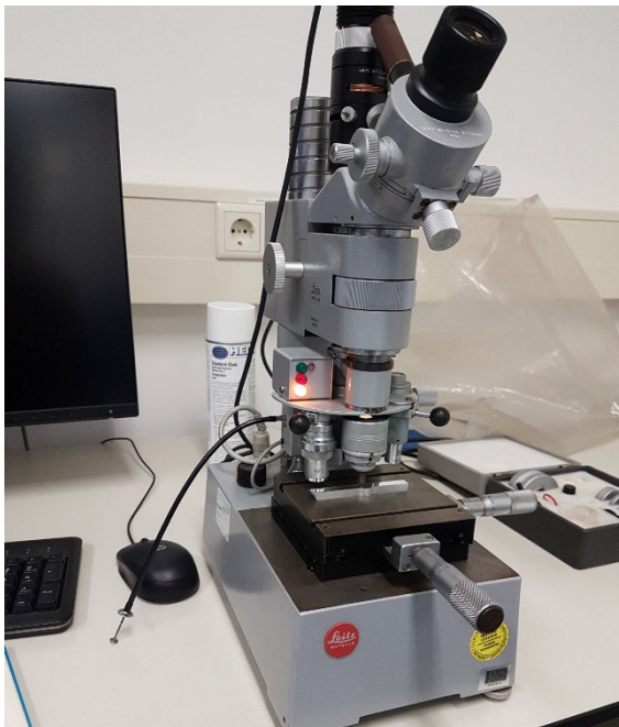
Figure 4.16: Leitz micro Vickers Hardness tester.
