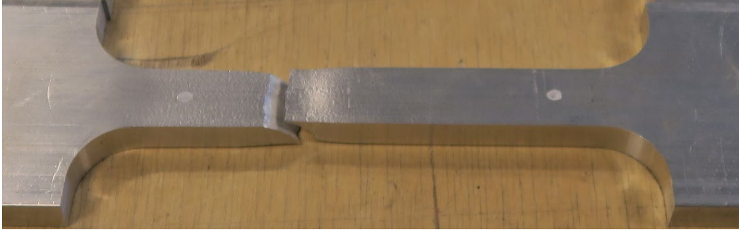
Figure 5.13: Failed base material specimen (BM.6.1).
