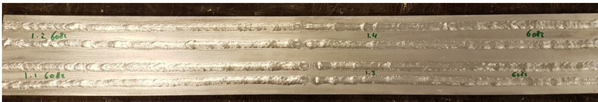
Figure 4.5: Picture of the longitudinally welded plate produced for dogbone specimens.
