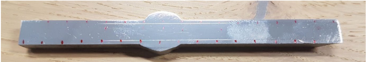
Figure 4.20: Prepared TW.6.3 specimen for measuring hardness.
