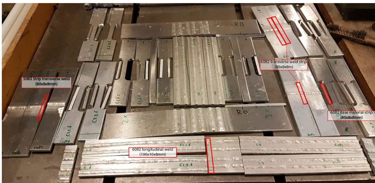
Figure 4.18: Cut out dogbones and indicated hardness specimens.
