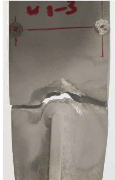
Figure 5.56: Picture of specimen W1-3 at the moment of complete failure.
