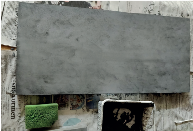
Figure 64: Adding pattern to concrete with colourant and sponge
