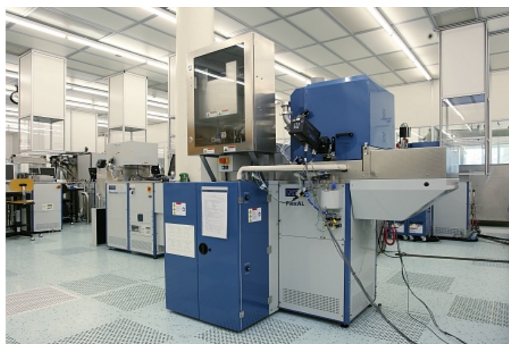
Figure 3.3: Picture of Oxford instruments plasma ALD system (FlexAL2) which is located in Nanolab@Tu/e [30]
