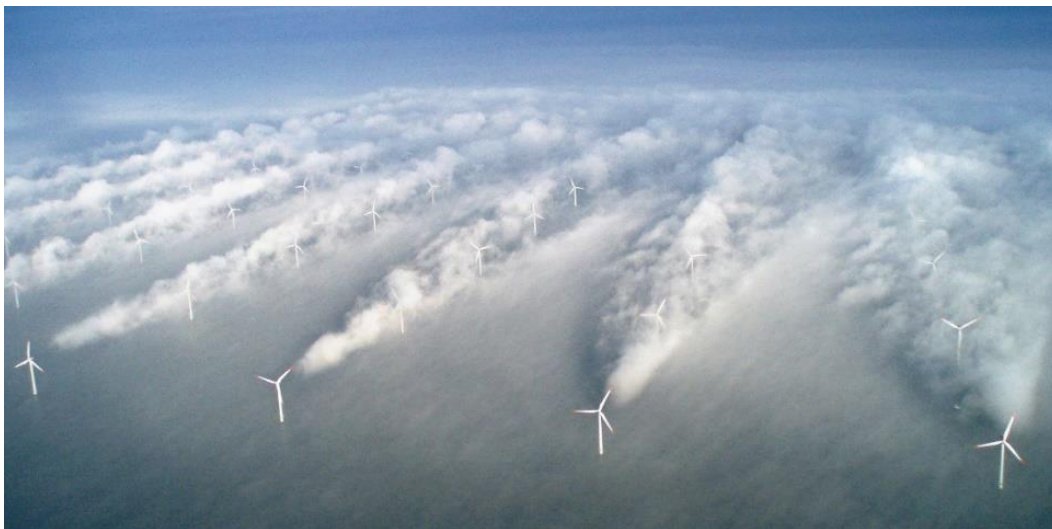
Figure 25: The wake effect behind turbines which is revealed by fog at Horns Rev wind farm in Denmark (Recharge, n.d.).
