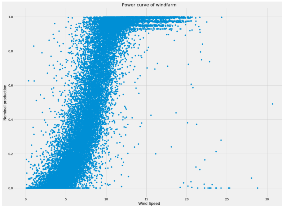
Figure 24: Power curve of one of the wind farms which shows the relation between the windspeed and the nominal production of the park.
