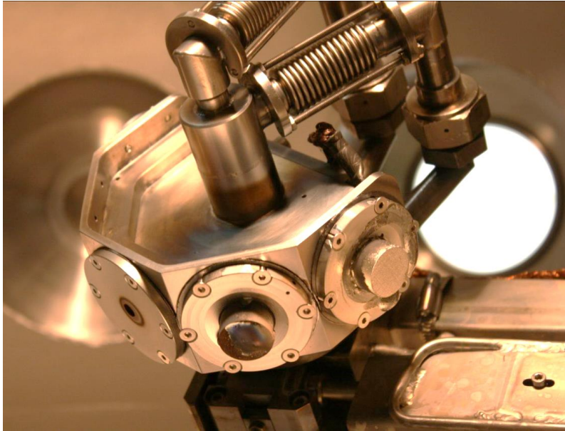
Figure 8-10 Target holder rotating inside the TEAC with the dummy (left), conventional (center) and V-shape (right) targets. This image was taken after the shot with trigger number 9689 (see Table 9-1 ). Conventional model had been exposed under a heat load of 18 \text{ MW/m}^2 and the V-shape under 25 \text{ MW/m}^2 . Notice the different colour of the targets in this image from the one they had before the exposure when the surface Li was oxidized (see Figure 8-8 ).
