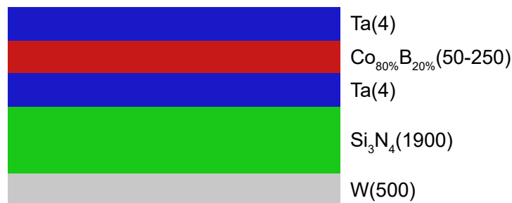
Figure 3.2: Schematic of the used material stack. The membrane that acts as substrate consists of W(500 nm) and \text{Si}_3\text{N}_4 (1900 nm). On top of this Ta(4 nm)/ \text{Co}_{80\%}\text{B}_{20\%} (50-250 nm)/Ta(4 nm) is deposited using magnetron sputtering.
