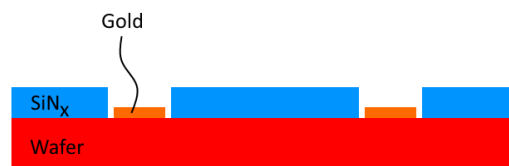
Figure 1: Schematic of a wafer just before the gold catalysed nanowire growth process.
