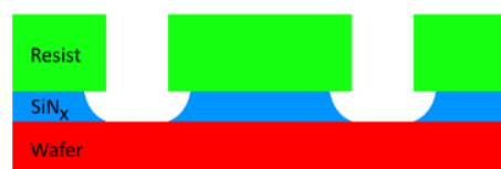
Figure 7: Sketch of wafer after wet etching process.
