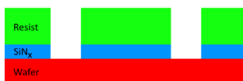
Figure 8: Sketch of wafer after dry etching process.
