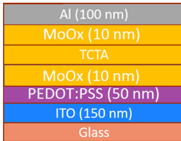
Figure 3.3: (a) Cross section of the matrix stack, (b) schematic energy level diagram of the matrix stack. In order of deposition which is from (a) bottom to top, (b) left to right, ITO, PEDOT:PSS, MoOx, TCTA, MoOx and aluminum, with thicknesses of 150 nm, 50 nm, 10 nm, various, 10 nm and 100 nm respectively.
