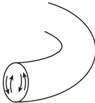
Figure 1.6: Zonal flows in a toroidal geometry. The arrows denote the flow directions. Adapted from [4].
