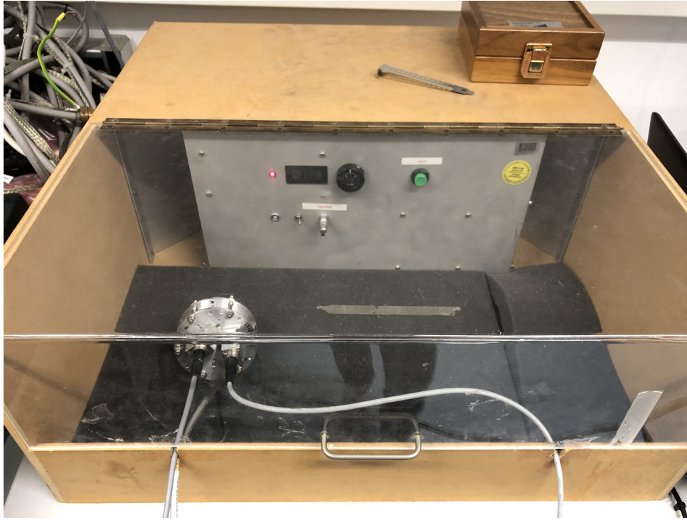
Figure 3.2: The cavity inside the temperature calibration device.
