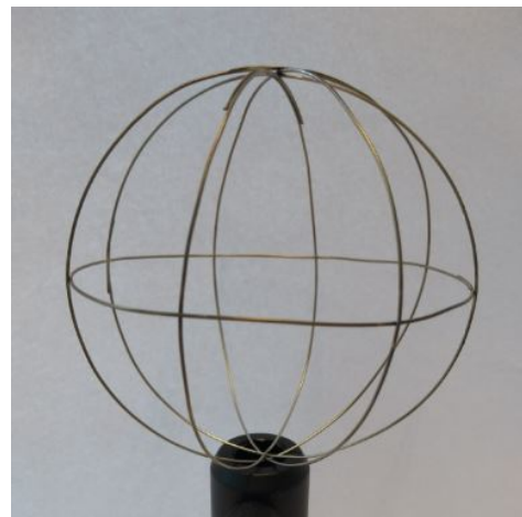
(b) The Nichrome grid with a radius of 4 cm, consisting of 5 wires.
