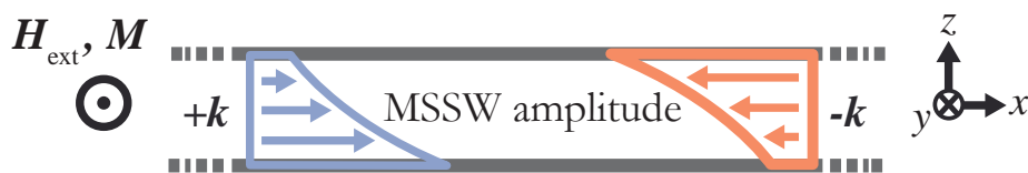
Figure 6.1: Side view of surface waves in a thin film, traveling perpendicular to the applied field H_{\text{ext}} . Blue and red regions represent the spin wave amplitude along the thickness of the film for waves traveling in the positive and negative x -direction, respectively.
