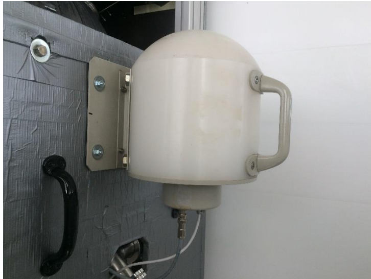
Figure 13: Studsvik 5310C neutron detector, mounted on the fusor at a distance of 48.7cm from the center.
