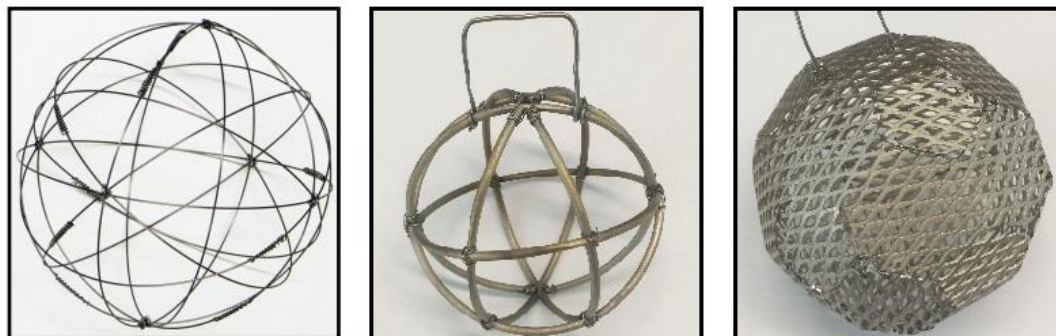
Figure 9: Different grid configurations used in this thesis. From left to right: 1) W wire grid \text{\O} 10\text{ cm} . 2) Ti wire grid \text{\O} 6\text{ cm} . 3) Ti mesh grid \text{\O} 8.5\text{ cm} .
