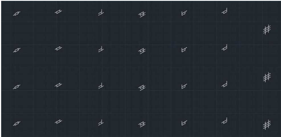
Figure 97: Autocad file of different designs used in this experiment. The designs are repeated 4 to 10 times above each other. The distance between designs is ten micrometer. Width, height, thickness and angle have been changed to examine the growth.
