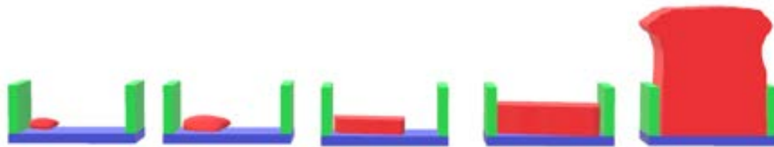
Figure 46: Illustration of a side view of a nucleation with the SiN mask in green, the InP substrate in blue and the InSb nucleation in red. The nucleation seems to start at the edge of the trench. If it gains a certain volume it forms visible favorable facets. The top of the nucleation is flat (111) direction. After a while the InSb can grow thicker than the SiN mask.
