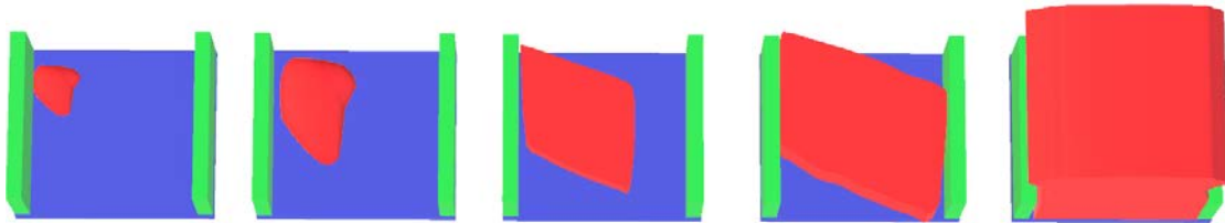
Figure 59: Illustration of a top view of a nucleation with the SiN mask in green, the InP substrate in blue and the InSb nucleation in red. Observe again the facets forming after some time and the nucleation starting at the edge. After some time the InSb can outgrowth the SiN mask and grows thicker than the trench width.
