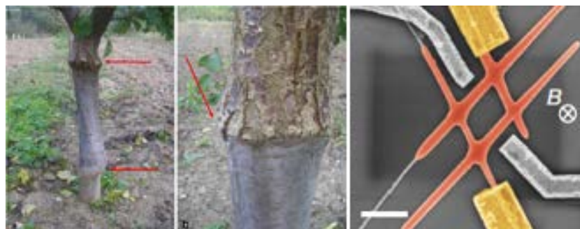
Figure 6: Final setup for the transport measurements. The loop is put down on a surface for contacting and gating. A magnetic field is applied perpendicular to the surface. Left images show the grafting of trees, comparable with the use of an InP stem.
