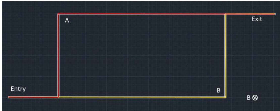
Figure 10: Autocad file showing the design of an AB-loop. One electron may move from entry to exit via A while the other one moves from entry to exit via B. While a magnetic field is applied perpendicular to the surface, this gives rise to an interference pattern.
