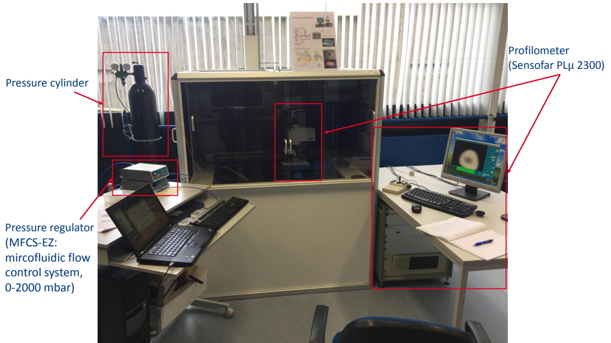
Figure 2.9: Experimental setup for bulge testing. The profilometer (Sensofar PL \mu 2300) is placed in a temperature and shock-proof chamber. Both the sample location, supplied pressure and measurement setup can be controlled from outside of the controlled chamber.
