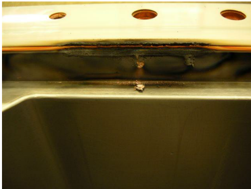
(a) Damage on the 150° left arc chamber plate and Mylar gasket. (b) Damage on the 330° left arc chamber plate.
