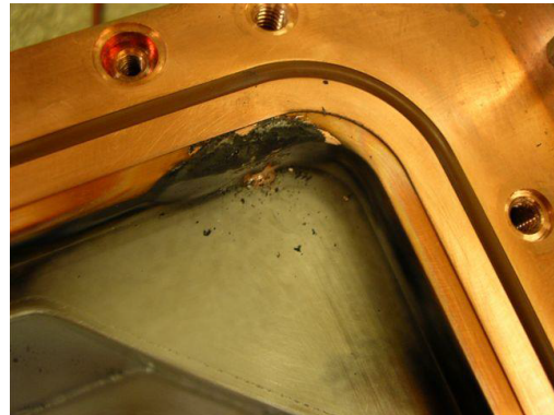
(a) Damage on the 150° left arc chamber plate and Mylar gasket. (b) Damage on the 330° left arc chamber plate.
