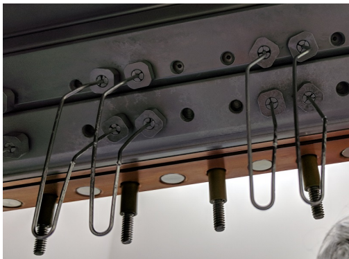
Figure 2.4: Detail of the degradation of four filaments after beam operation. The filaments are bent, and the surfaces pitted and rough. Various filaments are snapped in two.
