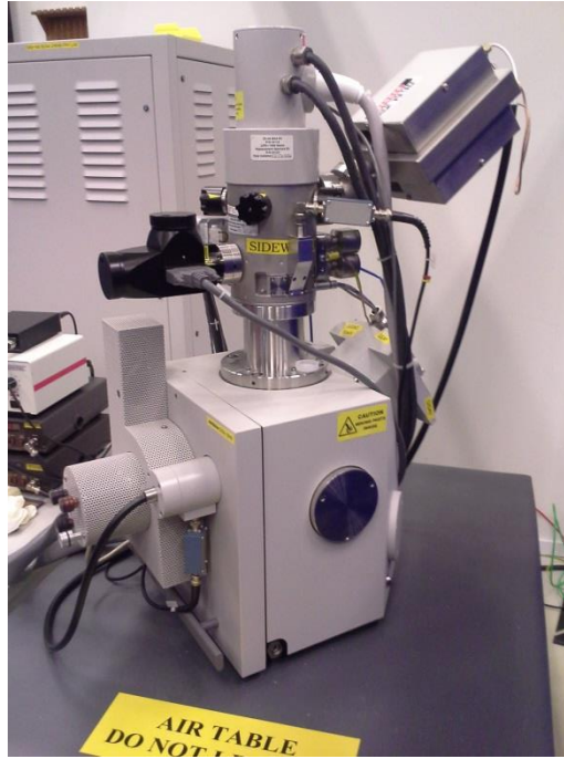
Figure 1.1.2: Picture of a Ga LMIS FIB. This particular FIB is the FEI FIB 200TEM used in the experiments detailed in Chapters 3 and 4 and is further described in Chapter 2.
