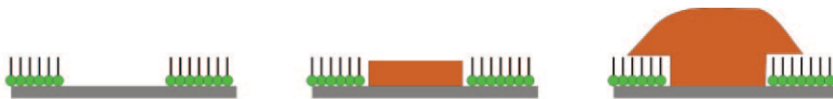
Figure 7.3: Illustration of lateral growth during area-selective ALD, resulting in a mushroom-like structure. 97
