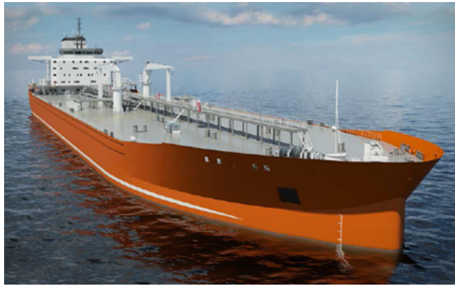
Figure 1.3: An Aframax tanker with a length of approximately 250 meters and a width of approximately 44 meters [17]
