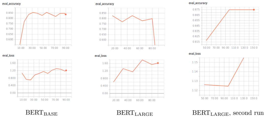
Figure 4.2: TensorBoard visualisation or ‘summaries’ for fine-tuning pre-trained models on AskUbuntu. Here the horizontal axis denotes the number of steps. Accuracy and loss for the model trained on the test set is evaluated at fixed steps on the evaluation set. The plots show that BERT is in some cases able to converge to a correct local minimum after 100 steps (3200 examples shown to model). The scores in these images should not be compared to the scores in Section 3.3.2 since the metrics and the data split differ.
