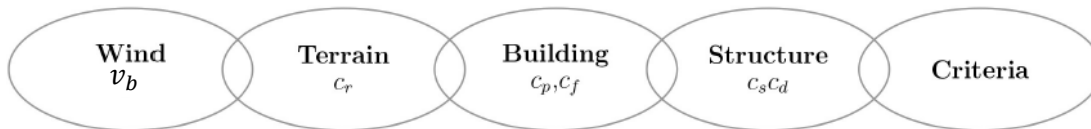
Figure 29 - Davenport wind loading chain
