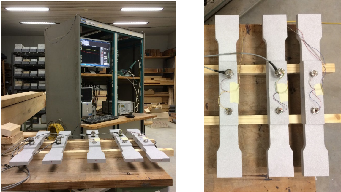
Figure 4.7.19: Test setup relaxation experiment instrumented bolts
