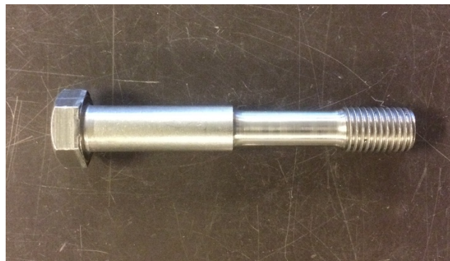
Figure 4.7.4: M16x110mm bolt with reduced shank used in tensile test
