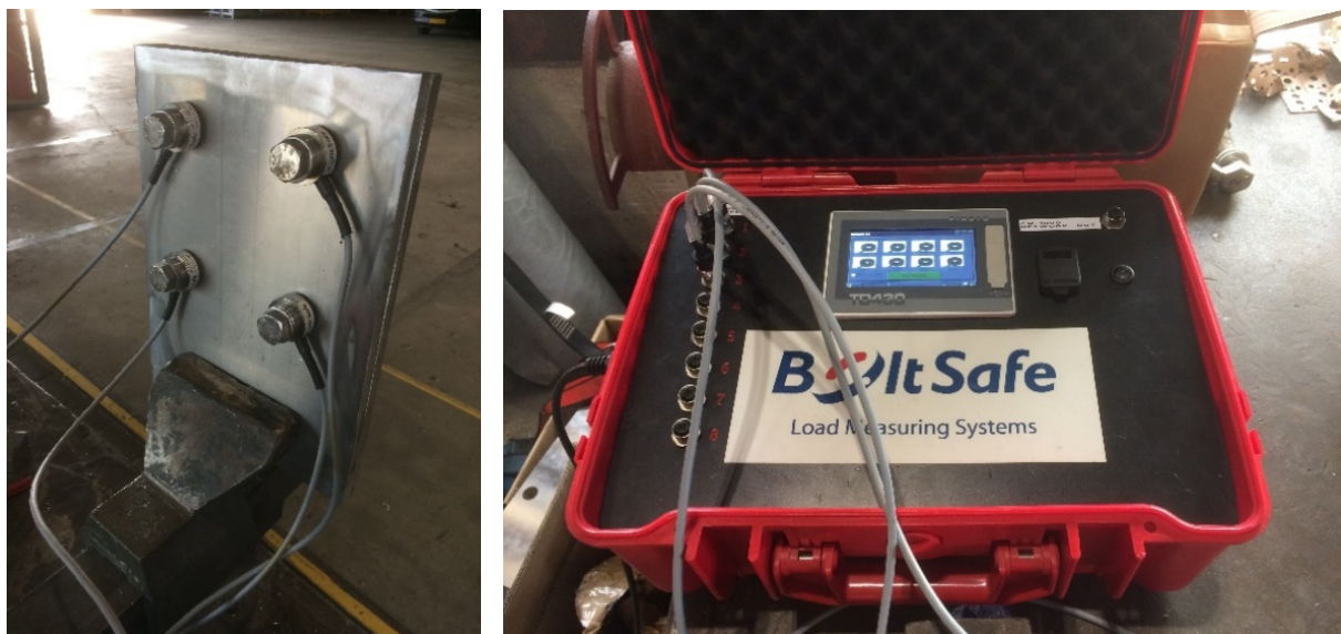
Figure 4.4.1: Test setup experiments torque – preload force
