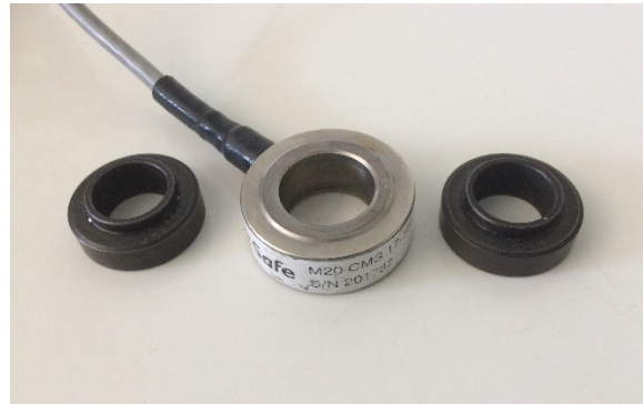
Figure 4.2.1: Bolt Safe Load Cell and Adapter rings
