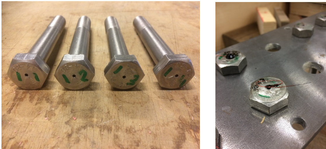
Figure 4.7.2: Bolts before (left) and after (right) installation
