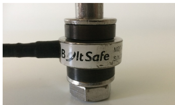
Figure 4.2.3: Side view Load Cell, adapter rings and additional washer
