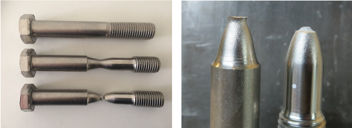
Figure 4.7.9: Necking and fracture of specimens (left) and detailed fracture (right)
