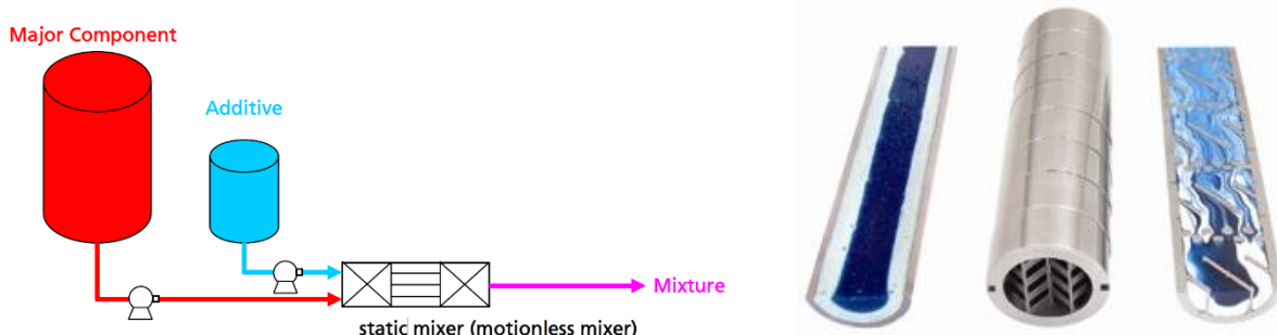
Figure 3-6 static mixing principle (left) and section of two liquids without and with static mixing elements (right). Both images taken from Stamixco Technical Bulletin [39].
