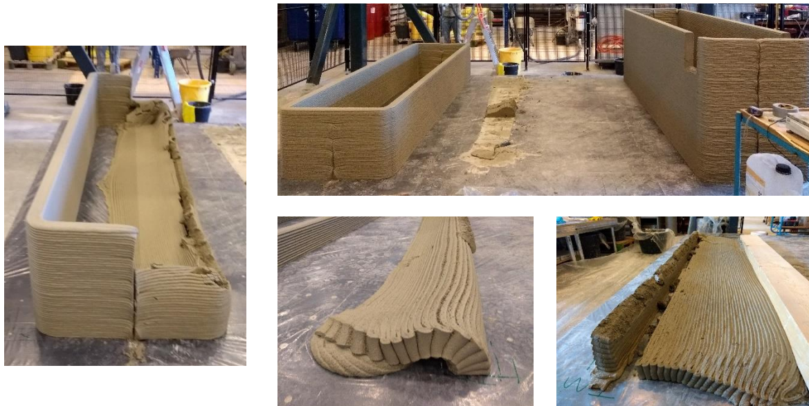
Figure 4-24 pictures taken during printing experiments. Left: rectangle printed without accelerator. Left and right part collapsed separately. Top right: difference between accelerated(right) and unaccelerated(left) rectangle, picture taken shortly before the collapse of the unaccelerated rectangle. Bottom: difference between accelerated(right) and unaccelerated(left) free-standing walls after failure.
