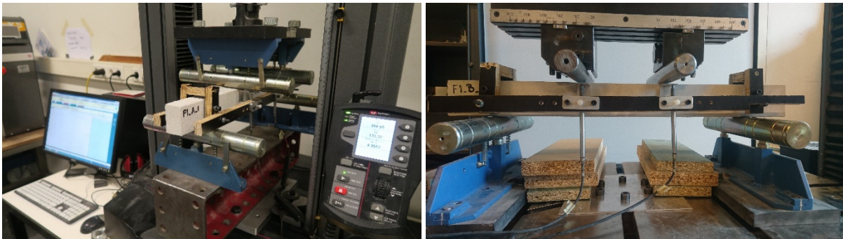
Figure 5.3: Test set-up four-point bending test; Overall set-up (Left); Location of LVDTs (Right).
