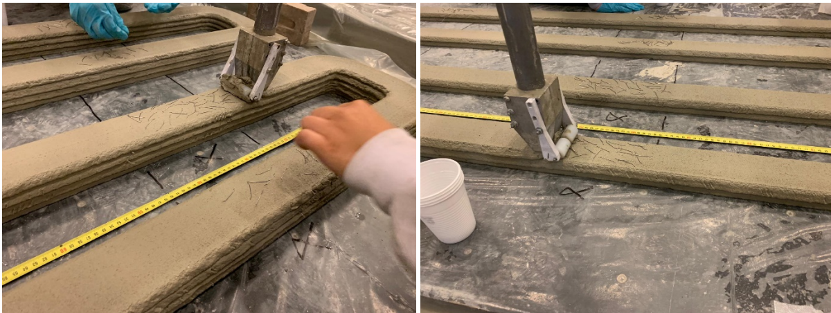
Figure 5.2: Specimen preparation, sprinkling of fibres by hand
