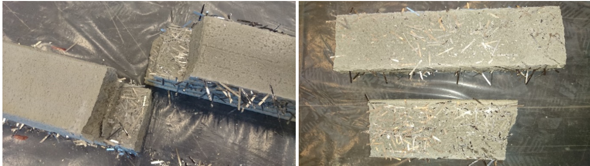
Figure 6.17: Failure in interface due to excessive overlap of fibres.
