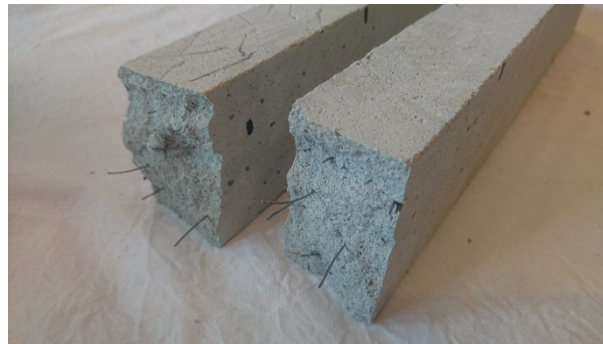
Figure 6.3: Straightening of hooked-end of Dramix 3D fibre.
