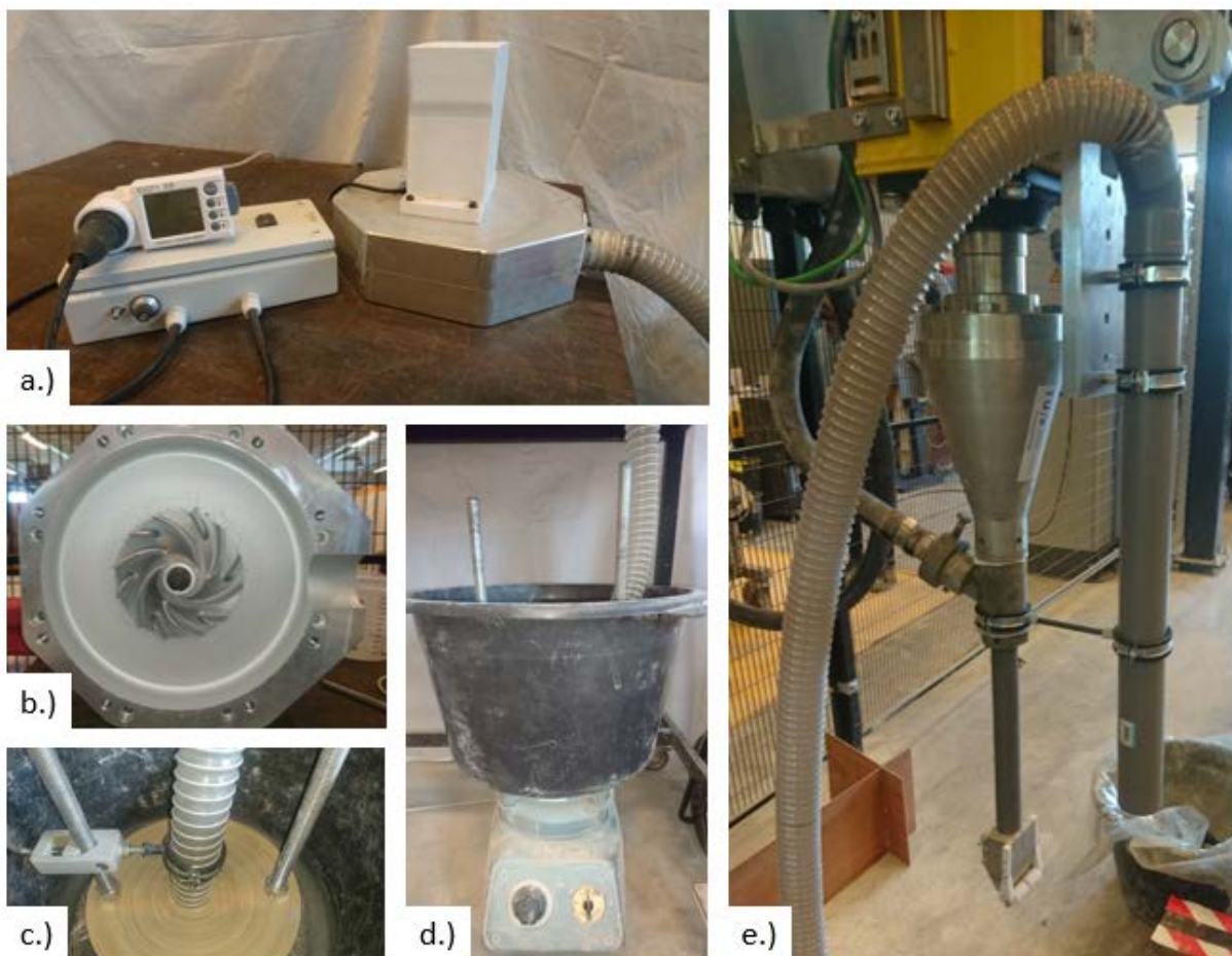
Figure 3.2: Final set-up of fibre blower; a.) Motor and wattage meter; b.) Rotor blade inside aluminium casing; c.) Fixation of input hose and funnel; d.) Vibration bucket; e.) Fixation of output hose at robot arm.
