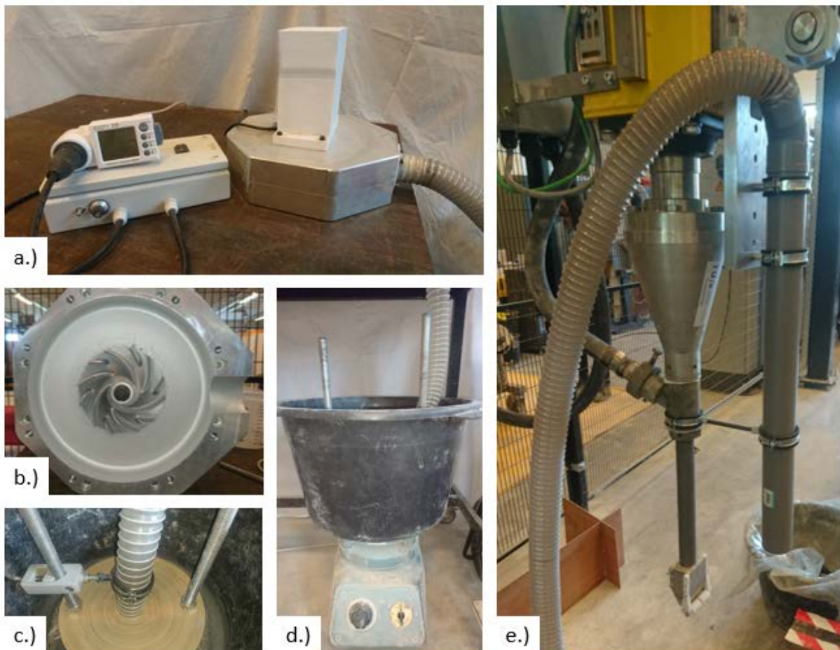
Figure B.2: Final set-up of fibre blower; a.) Motor and wattage meter; b.) Rotor blade inside aluminium casing; c.) Fixation of input hose and funnel; d.) Vibration bucket; e.) Fixation of output hose at robot arm.
