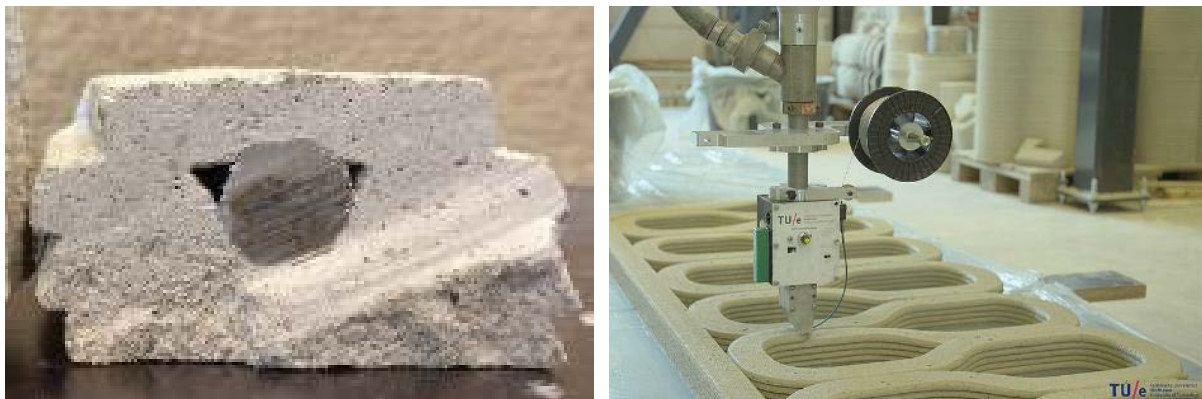
Figure 1.2: Section of rebar in printed concrete (Left); Printing of cable reinforced concrete (Right). (Goris [19]; Dezaire [15])
