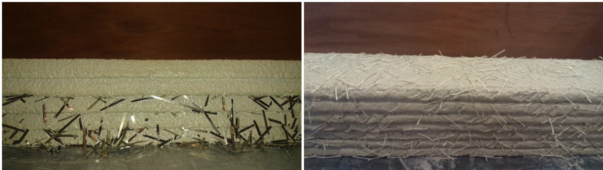
Figure B.20: Fibres on sides of printed element.
