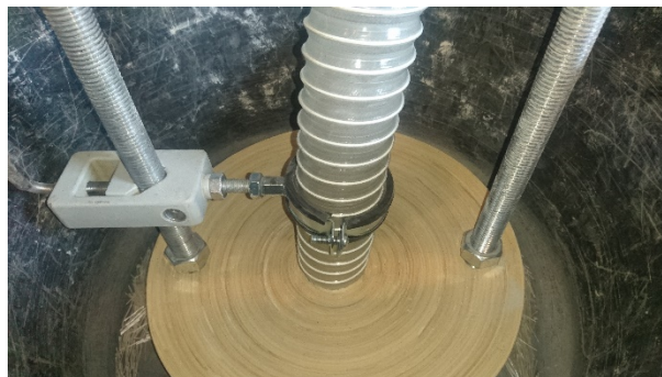
Figure B.9: Fixation of input hose in vibration bucket.
