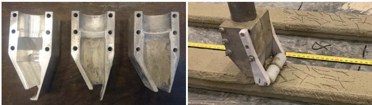
Figure 3.12: Different nozzle types used at the Eindhoven University of Technology; Back-flow nozzle; Hybrid nozzle; Down-flow nozzle; Roller attachment (From left to right).
