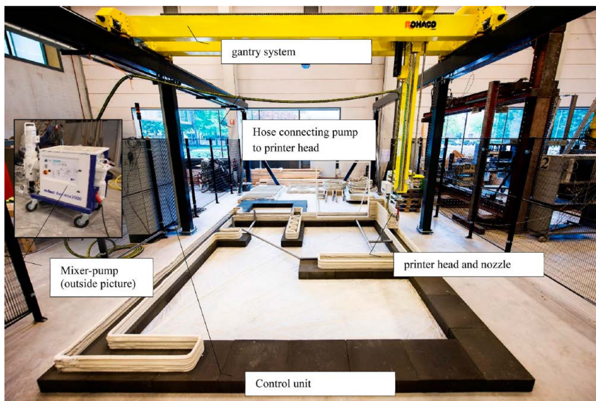
Figure 1.1: 3D Concrete printing facility at the Eindhoven University of Technology. (Bos et al. [7])
