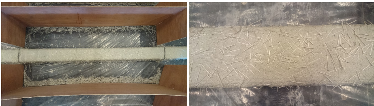
Figure B.18: Fibre distribution over print path for Cem-FIL Minibars 24mm.
