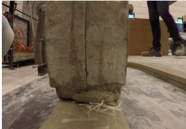
Figure 3.15: Scraping of fibres by using a hybrid nozzle.
