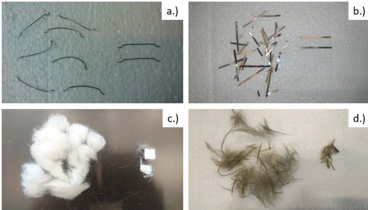
Figure B.4: Deformation of fibre types due to rotor blade; a.) Dramix 3D RC-4530-BL; b.) Fibraflex FF/30L6; c.) Duomix M12; d.) Uncoated chopped fibres.
