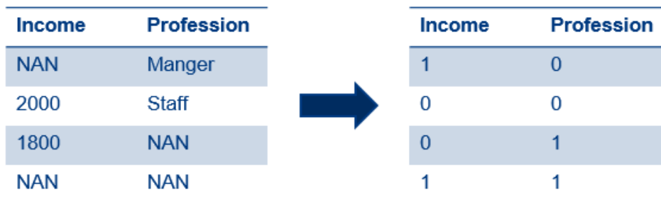
Figure 4.12: Occurrence of missing values denoted as 1, otherwise 0
