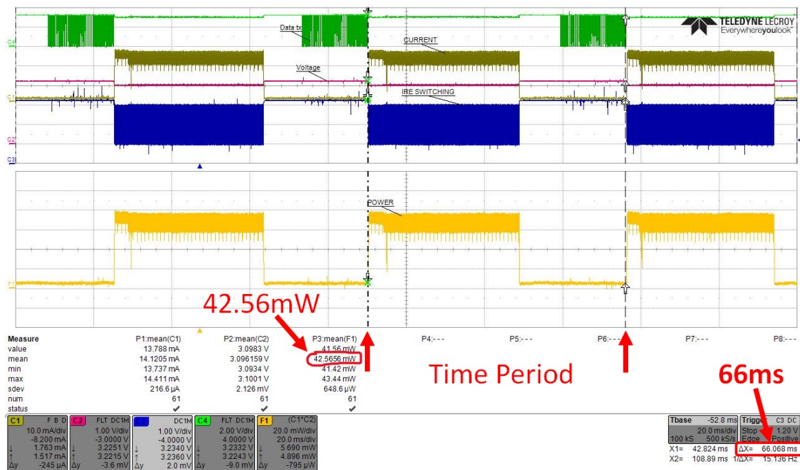
Fig. 7.9 Reduced mean power consumption by 38.64mW or about 48% with pulse synchronised power saving scheme.
