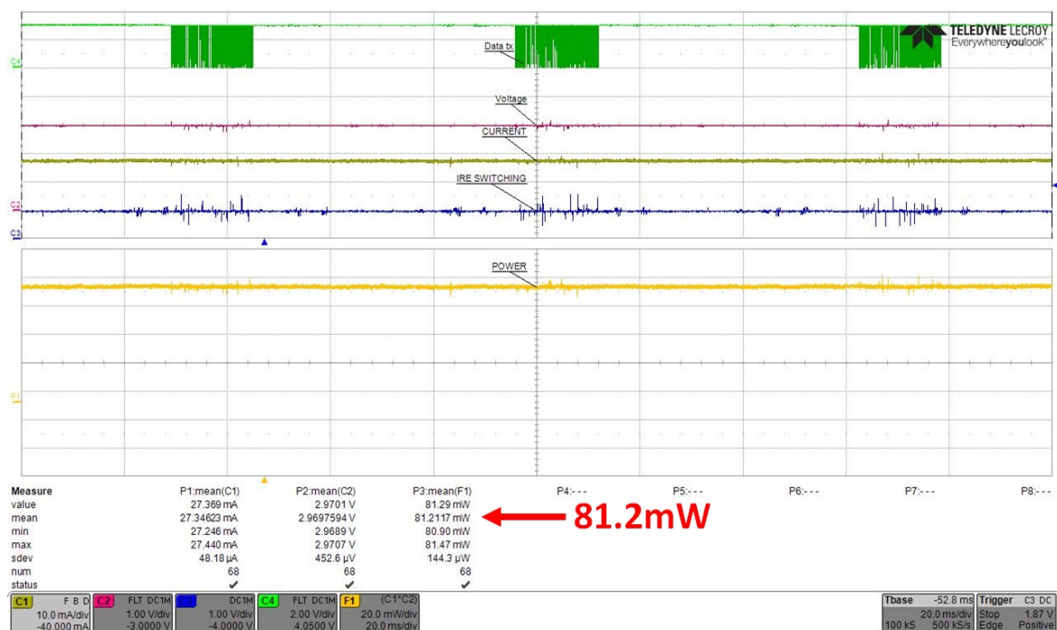
Fig. 7.8 Mean power consumption of 81.2mW without pulse synchronised power saving scheme.
