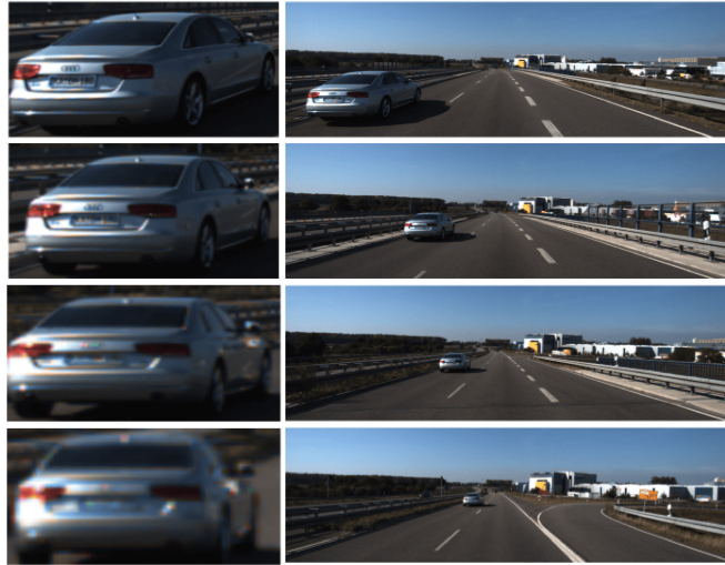
Figure 3.7: Left: cropped images of a car. Right: Images of the whole scene. The local orientation changes in different images while the global orientation remains the same [20].
