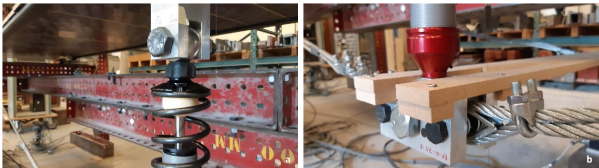
Figure 6.29: Application of dampers in the bridge model: top detail (a) and bottom detail (b)
