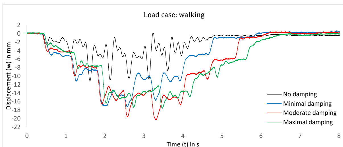
Figure 6.31: Walking over the bridge: experimental measurement at center span
