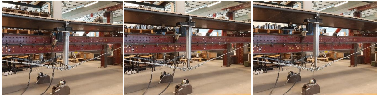
Figure 6.23: Changing the set point in the Labview script to generate different values for stiffness of the cable truss.
