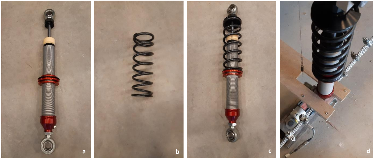
Figure 6.27: Viscous damper (a), spring (b), shock absorber (c) and application in bridge (d)
