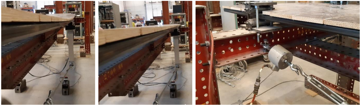
Figure 6.7: Bridge without (a) and with pretension in the cables (b) and measuring the cable pretension (c)
