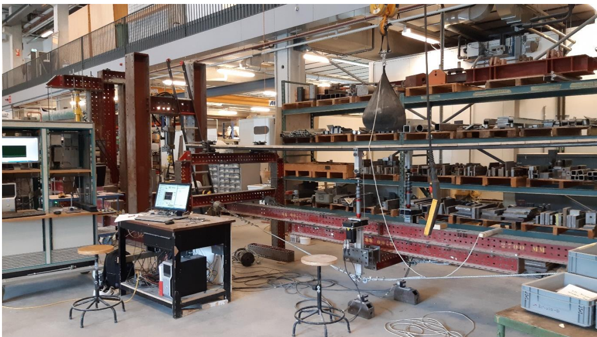
Figure 7.1: Test setup for the controlled impact test at center span
