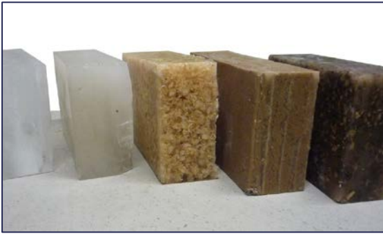
Figure 2; Different samples of reinforce ice (Janssen, et al., 2013)
