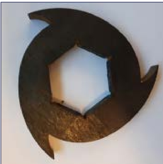
Figure 82; Engineered and watercutted shredder tooth
