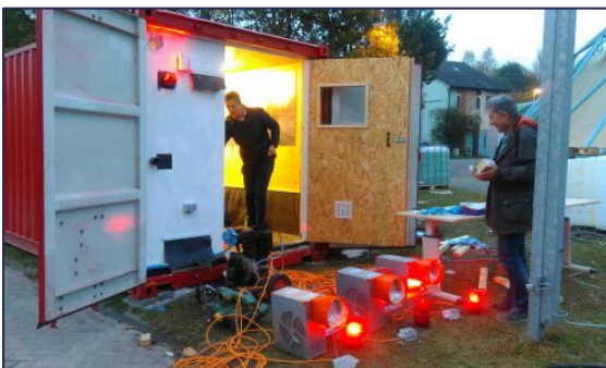
Figure 109; Test of the air monitoring system with acoustic and visual alarms
