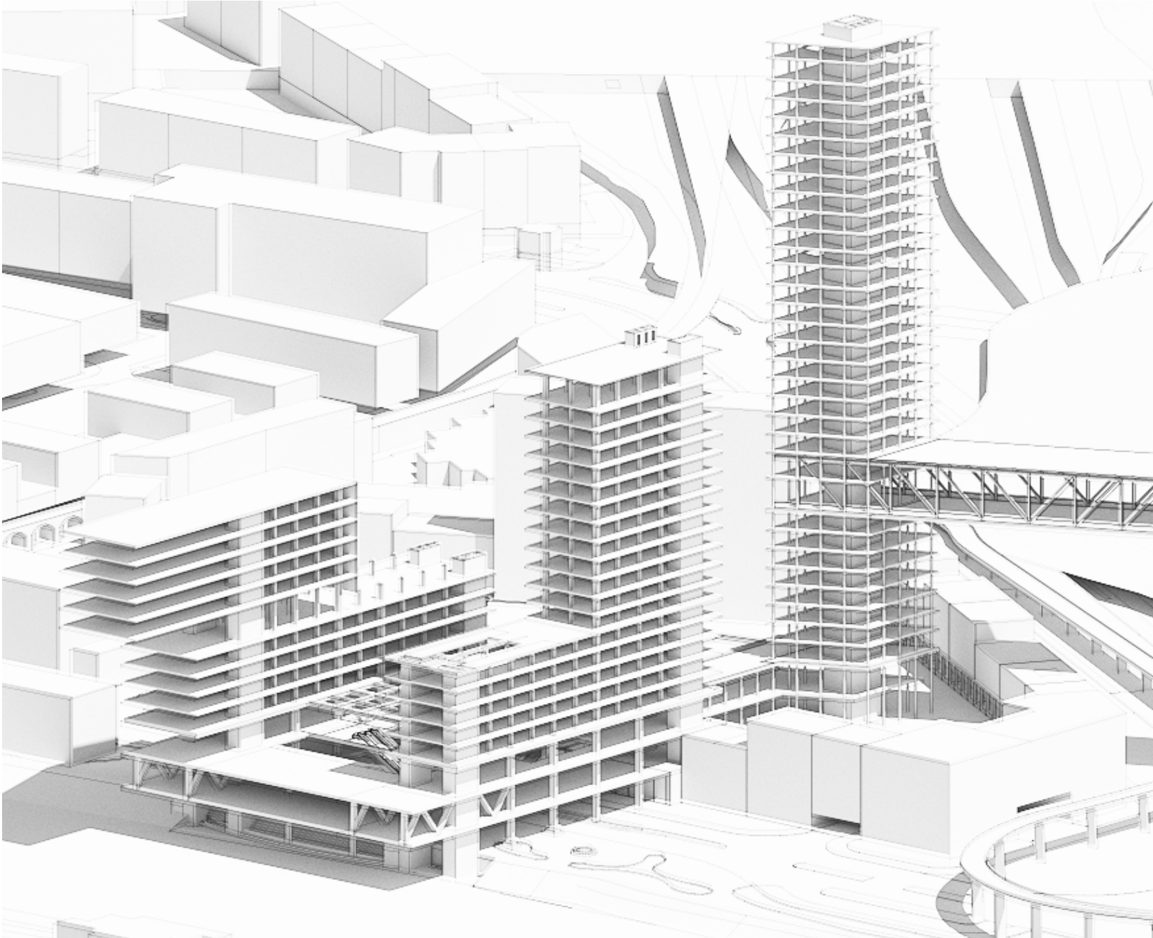
An overview of the concrete and steel (truss) structure
