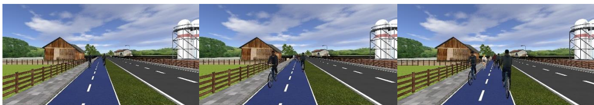
-Figure 13: Intensity levels of cyclists: low (1000 cyclists/h), medium (2500 cyclists/h) and high (4000 cyclists/h)
