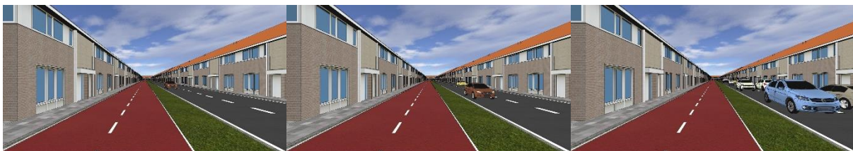
-Figure 18: Intensity levels of car traffic: low (250 cars/h), medium (1000 cars/h), high (2000 cars/h)
