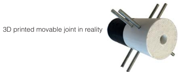
fig.4.23 Applying the 3D printed movable joint from the research of 3DCP of fellow students which focused on Joints. This will be fastened inbetween each block with steel nuts and bolts. © 3DCP research groups (2018)
