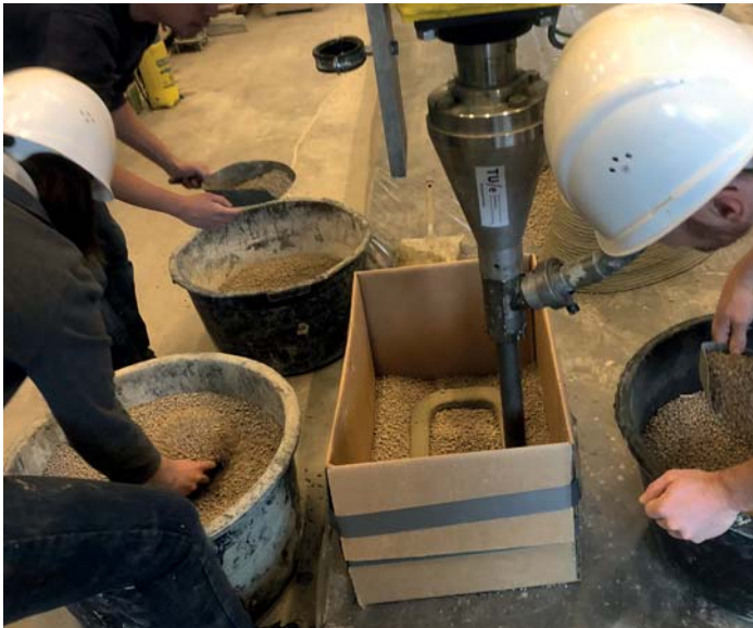
fig.1.6 Printing and filling it up layer by layer - in order to still be able to print several layers at once, and to achieve the actual height of the blocks, a box has been placed around the block where the inside and around the block is filled layer by layer. This filling keeps the curve and will not fall over.
