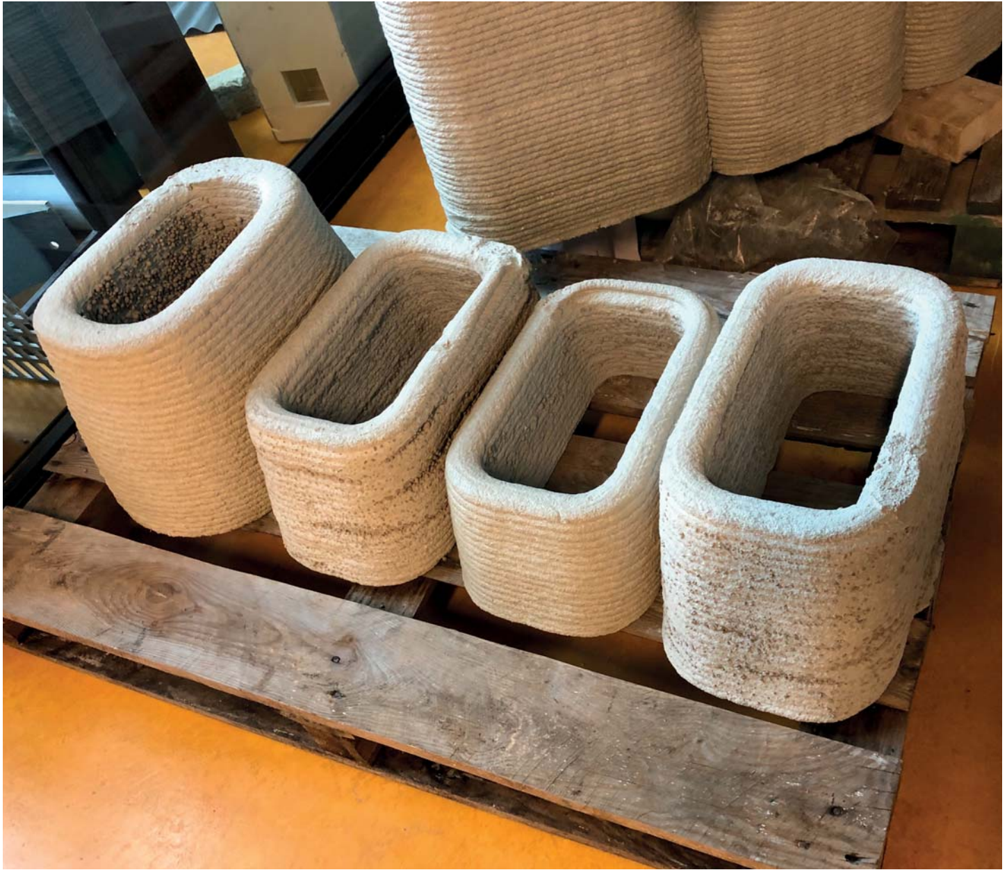
fig.1.8 The final result - after hardening and cleaning, the blocks are ready to be stacked to become a special tower. However, there are still filling materials on the inside of the blocks that have entered in the concrete, during printing and are hardened. These are not / difficult to clean. I also think that the structure of the filling material has an aesthetic value in the blocks, these therefore remain. A special process that I eventually became happy at the end.
