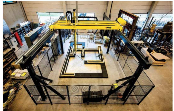
fig.3.3 3DCP at TU/e made of a four-axis gantry robot and features a print bed of 9.0m × 4.5m × 3m with its own mixing pump and controlled by a numeric controller. © Photo by Doomen
