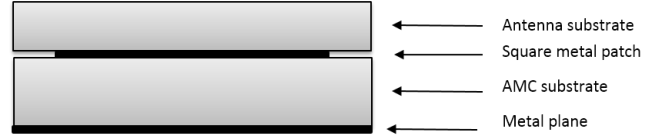
Fig. 5: Cross-section of the AMC unit cell (HIS plus the antenna substrate)
