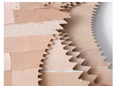
Figure IX.4. Custom lamination of plates results in varying stiffness over the length of the elements.
