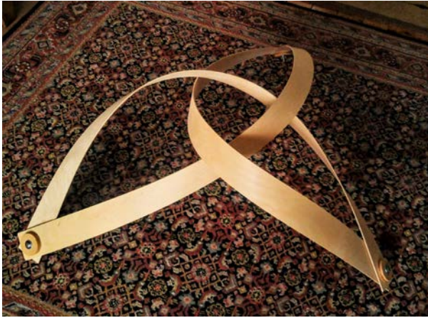
Model constructed from 3 bent plywood strips with the grain direction parallel to the longitudinal direction.
