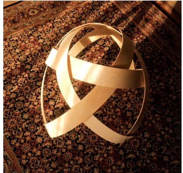
Model constructed from 4 bent plywood strips with the grain direction perpendicular to the longitudinal direction.
