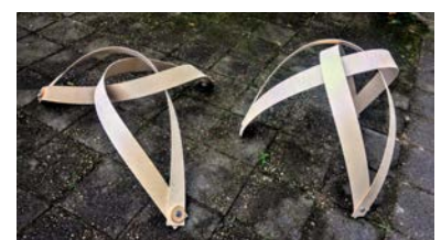
Figure 3.2. Two models constructed by the author with two sets of strips with the fibre direction oriented parallel (left) and perpendicular (right) to the longitudinal axis. The left model behaves significantly stiffer.
