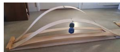
Figure 6.1. Simple load tests on the hinged (top) and clamped (bottom) system.
