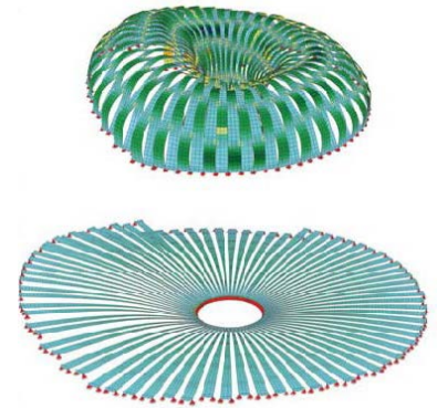
Figure 4.2. Contracting cables simulate the bending in the computation of the 2010 ICD/ITKE research pavilion (Lienhard, 2014, p. 69).
