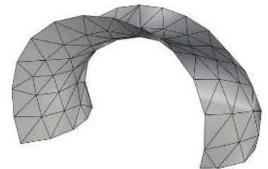
Figure VII.2. A triangular mesh is used to approach the curvature of the system.
