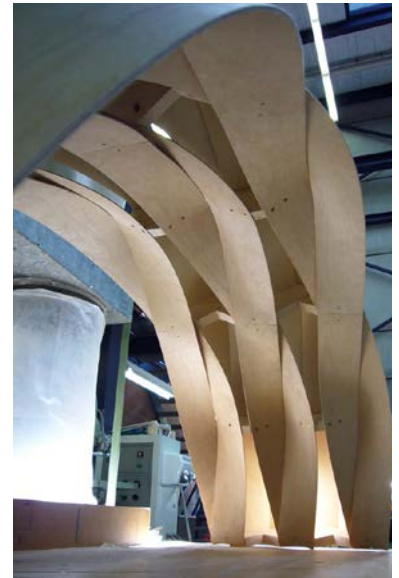
Figure IV.1. Prototype of the Timberfabric system.
