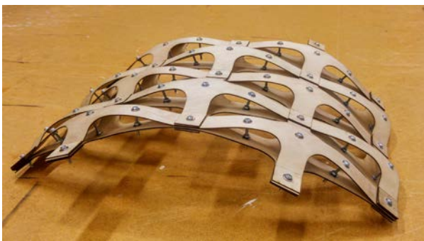
Construction sequence of a scale model of the modular system with 2 units in the longitudinal direction.
