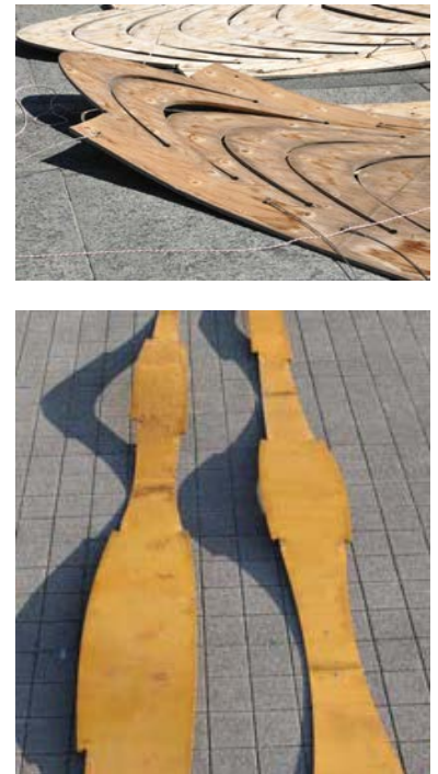
Figure 2.9. Plastic deformation as a result of stress-relaxation in the elements of the dismantled AA/ETH pavilion (top) and 2010 ICD/ITKE pavilion (bottom).
