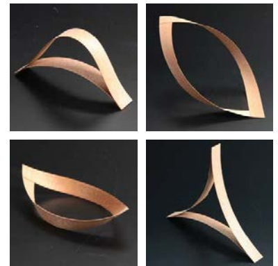
Figure 3.5. Systems with parallel connections (Lienhard, 2014)
