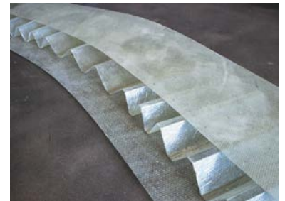
Figure XI.3. The multi-layer arrangement increases the stiffness but still allows the bending.
