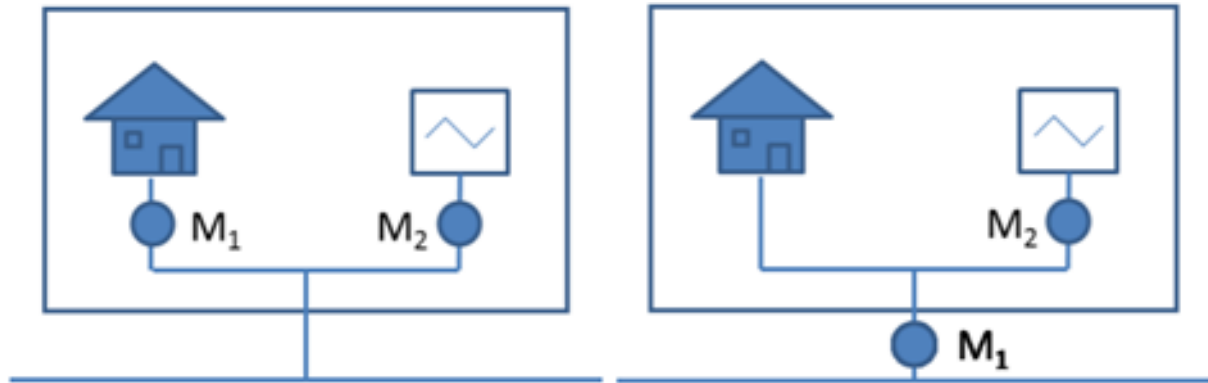
Figure 16 Diagram of connection with parallel (left) and serial (right) metering. M1 and M2 represent the two transfer points with the metering devices (ACM, 2016).
