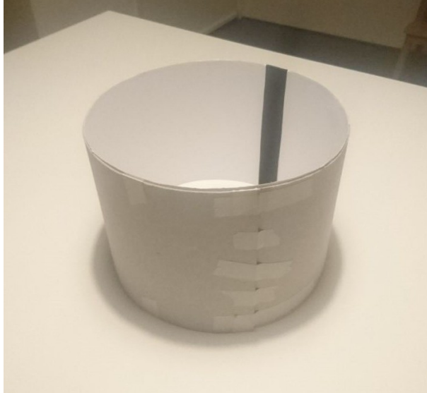
Figure 12: The cardboard cylinder with a test environment illuminated from above.
