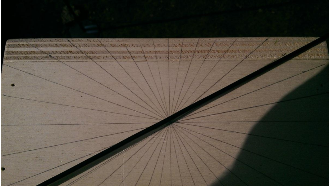
Figure 4.7 Photo of the wind rose on top of the big box used to aim the speaker
