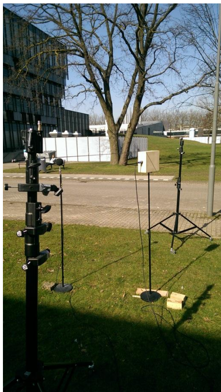
Figure 4.6 Photo of the set-up directivity measurement
