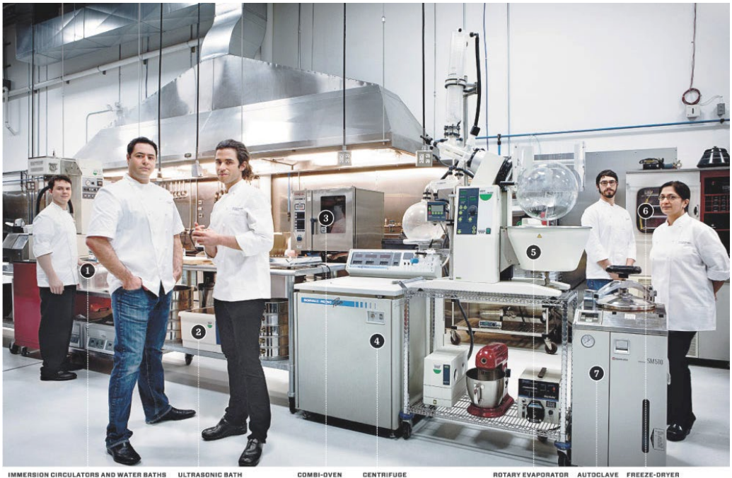
Figure 4.5 Molecular Gastronomy appliances. IMMERSION CIRCULATORS AND WATER BATHS ULTRASONIC BATH COMBI-OVEN CENTRIFUGE ROTARY EVAPORATOR AUTOCLAVE FREEZE-DRYER
