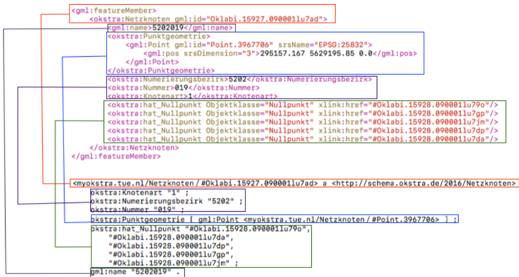
Figure 4.9: An Example of Transformation for OKSTRA XML to RDF
