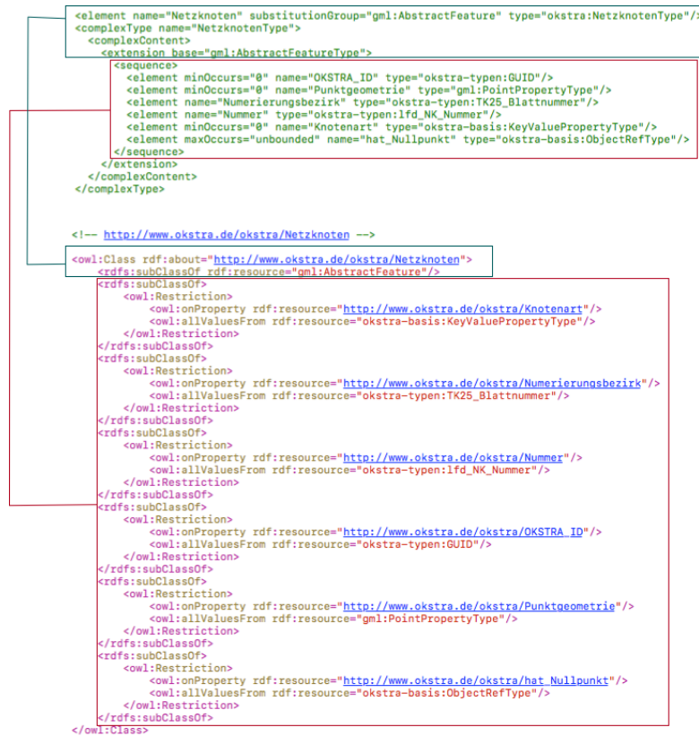
Figure 4.8: The Original XSD and OWL of OKSTRA Class 'Netzknoten'
