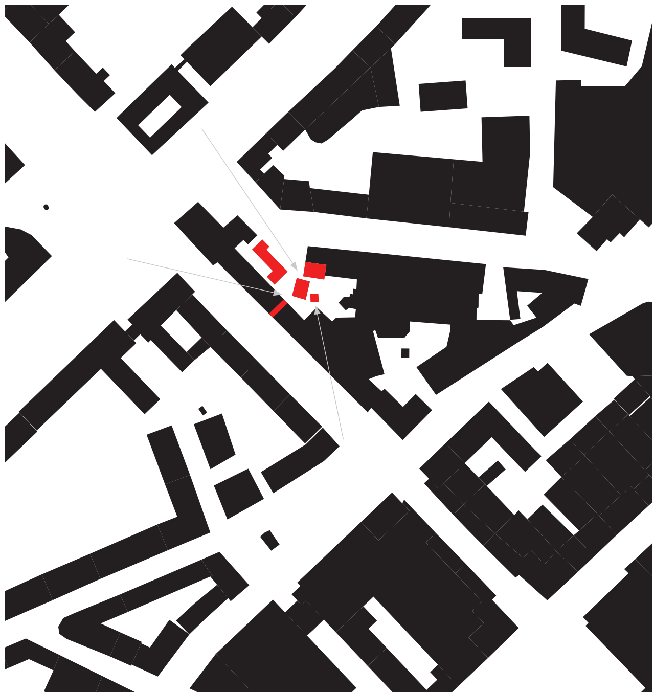
Fig. 72 The interventions shown in red, several volumes added in the location following the zig-zag pattern already present in the block, and a passage from the Treppenstraße into the area, creating a more permeable block and city structure.
