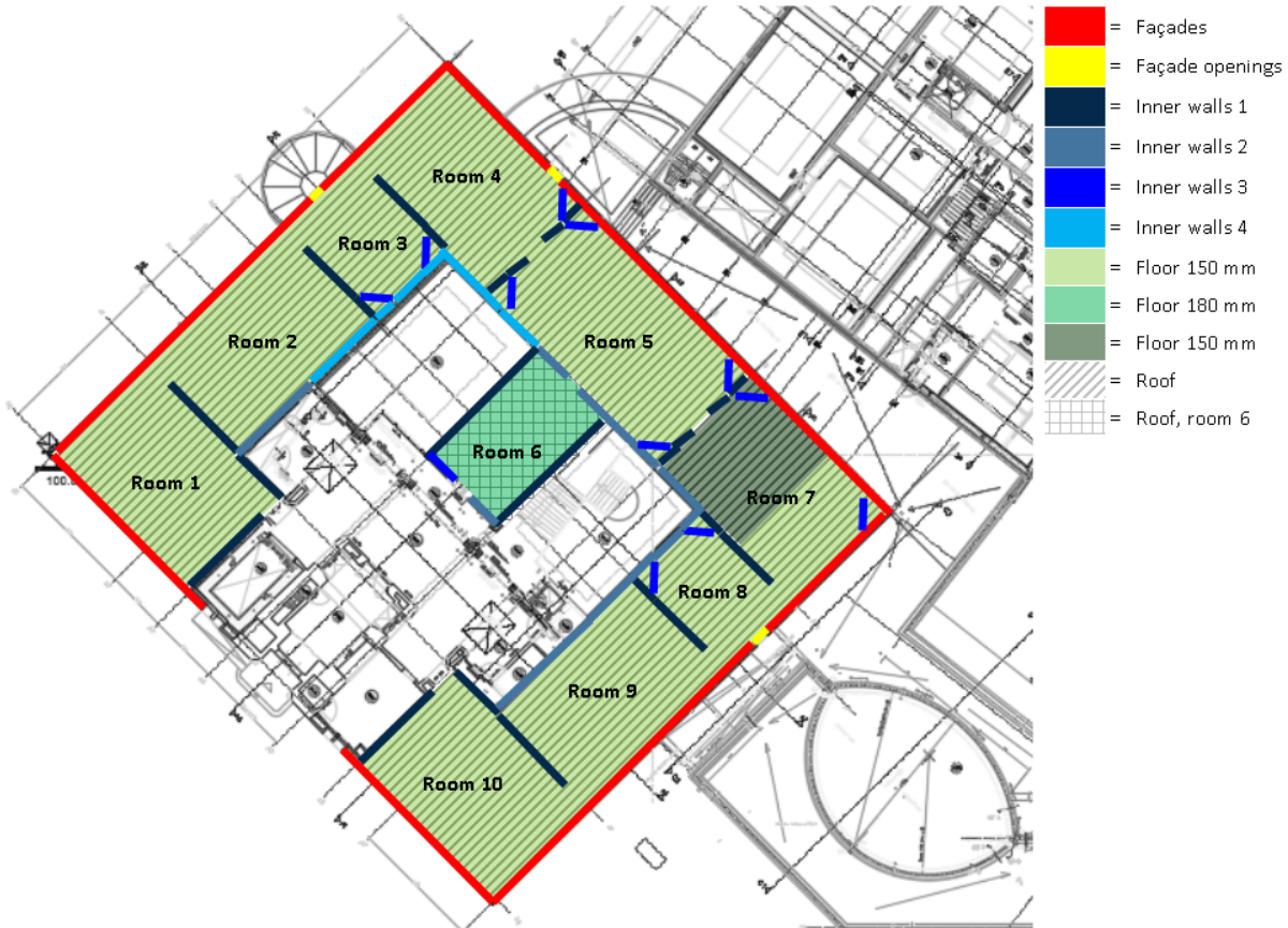
Figure 9.9: Structure types monumental building part A, floor plan under layer by Cahen (2003). All the walls of exhibition rooms have an extra double wall with a layer of multiplex and plasterboard.
