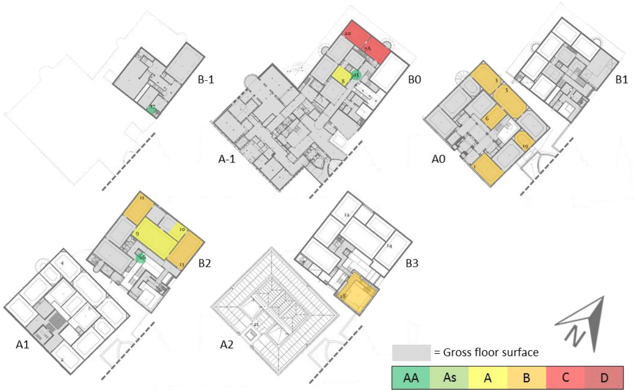
Figure 9.100: Best ASHRAE classes met 100% of the time, based on general climate risk assessment, during the total measurement period, floor plan under layer by Cahen (2003).
