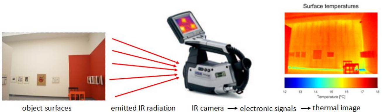
Figure 3.1: Principle of IR thermography. IR camera (Flir systems, 2004) detects the IR energy (heat) that a surface emits (the higher T , the higher the emitted IR radiation) and transforms it into electronic signals. These signals are converted to a thermal image (Flir, 2016)
