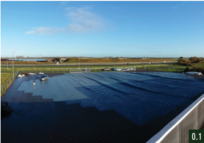
Production of the inflatable (2500 m 2 , 1600 kg) at Poly-Ned BV, Steenwijk Netherlands.
