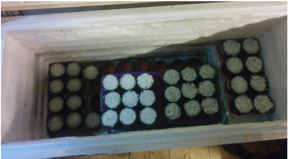
Figure 9: Frozen cellocrete samples prepared for testing
