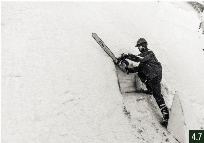
Cutting cellocrete blocks from the Bridge, for testing in the laboratory
