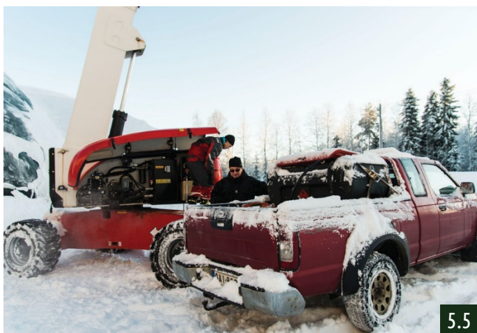
Filling boom lifts with gasoline
