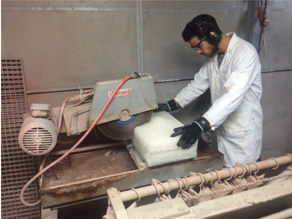
Figure 83: Sawing blocks of cellocrete at the laboratory
