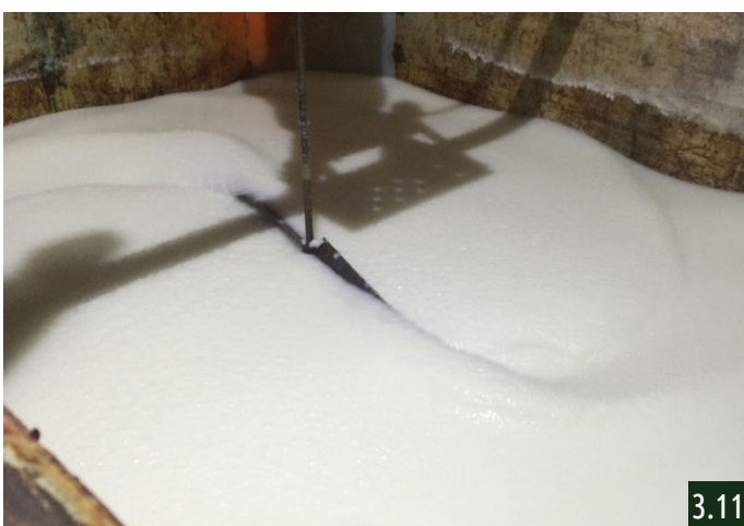
Mixing the cellulose fibers to a homogeneous 2% fiber weight ratio mixture
