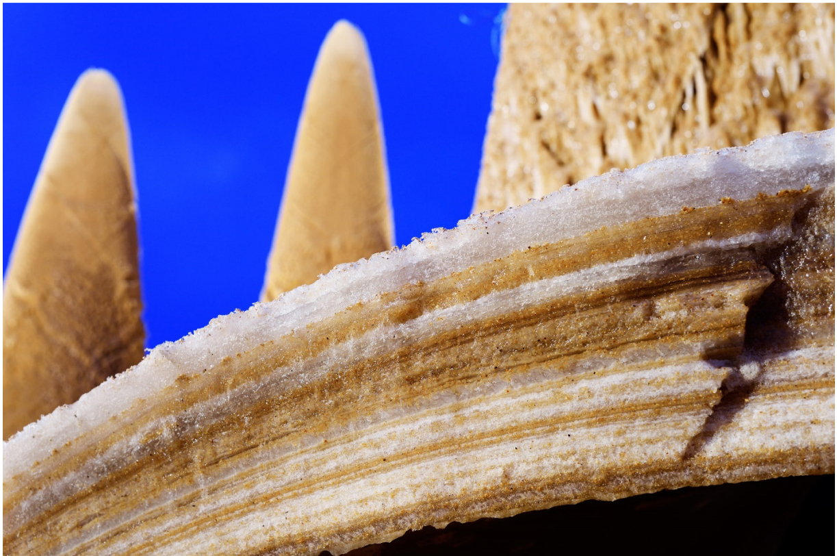
Figure 2: Layered pykrete section of Sagrada Familia in Ice (Photo: Bart van Overbeeke)
