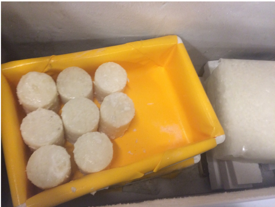
Figure 78: Cut cellocrete samples, prepared for testing
