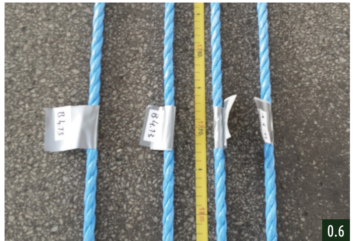
Measuring, labeling and cutting approximately 3 km of propylene rope
