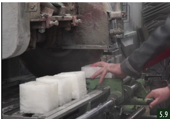
Sawing cellocrete blocks of 100x100x100 mm, with the machinery of the Tulikivi Stove factory.
