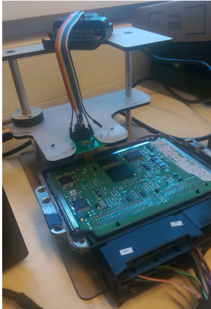
Figure 9.1: The ECM from model C, with the Multilink FX on-chip debugging tool connected to the BDM debug pads.
