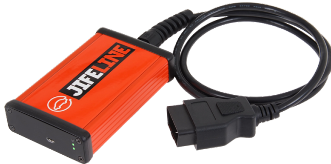
Figure 5.1: The Jifeline tool. It can be connected to a tablet using USB-OTG, which then forwards the CAN data over wifi. This allows for easy analysis as well as the possibility to interact and inject frames using Python.
