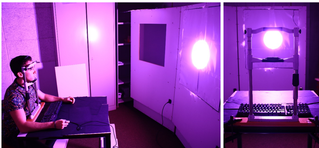
Figure 3.16: The stimuli was observed from a fixed distance of 150 cm, in a seated position and through the chin rest. Some reflective surfaces like the table, were covered with black thick paper.
