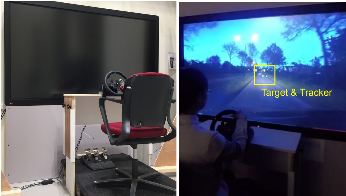
Figure 3.5. Photos of the driving simulator. The left figure shows the experimental setup, the right figure is a demonstration of the driving simulation. The target and tracker are marked with the yellow frame
